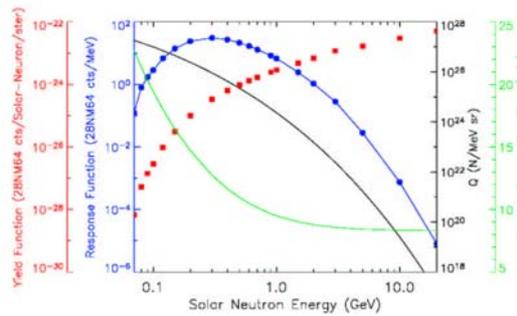
Figure 4. Yangbajing 28-NM-64 yield function versus energy for neutrons arriving 51degree from zenith (red squares), Chupp's [3] exponential spectrum (black curve), Yangbajing response function (blue), and propagation time of a neutron from the Sun to 1 AU (green).
